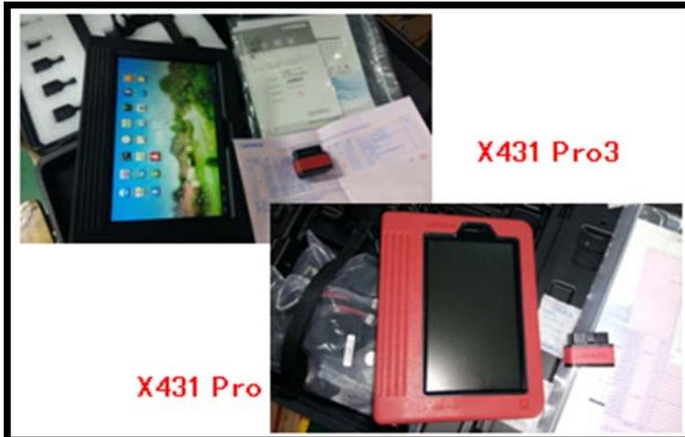
Feedback from Mr. Zhao (1398538\*\*\*\*) in Guizhou, Toyota Reiz, VIN=LFMBE22D7A0\*\*\*\*\*, 5GR Engine, 2010, see Picture 1. This car has changed the steering wheel. Torque sensor learning is successfully done by the X-431 PRO.
