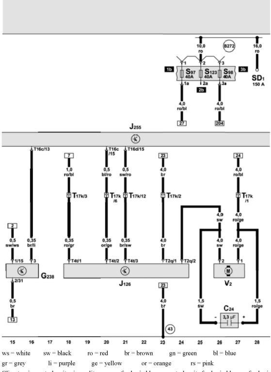
Climatronic control unit, air quality sensor, fresh air blower control unit, fresh air blower, fresh air blower fuse 1 and 2
