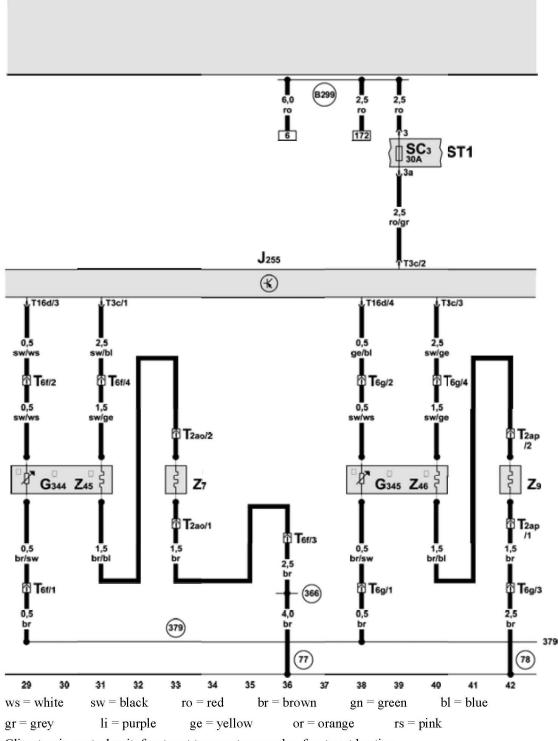
Climatronic control unit, front seat temperature sender, front seat heating
