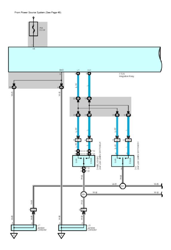
D 9 Door Key Lock and Unlock SWFront RH Door Lock Motor Front RH Door Unlock Detection SWFront RH
