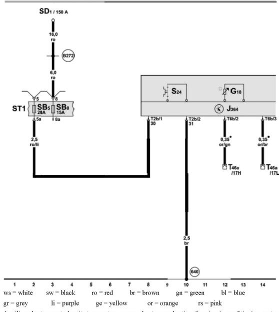
Auxiliary heater control unit, temperature sensor, heater overheating fuse in air conditioning system compressor
