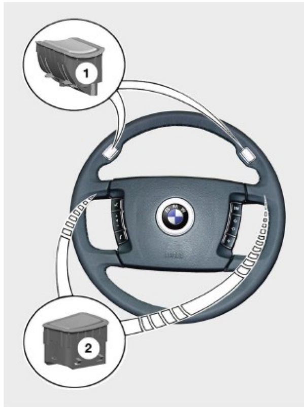
Fig. 15: Steptronic push-buttons in the MFL
