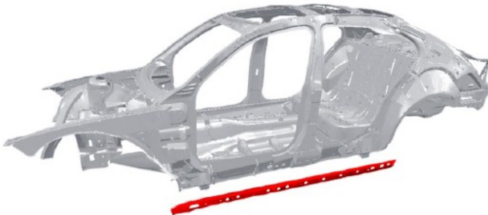
Fig. 11: Reinforcement profile section
